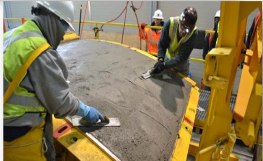
Segment being hand finished prior to demolding
