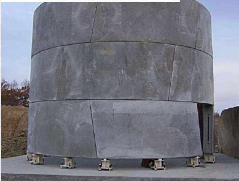
Segmental liner test ring build
